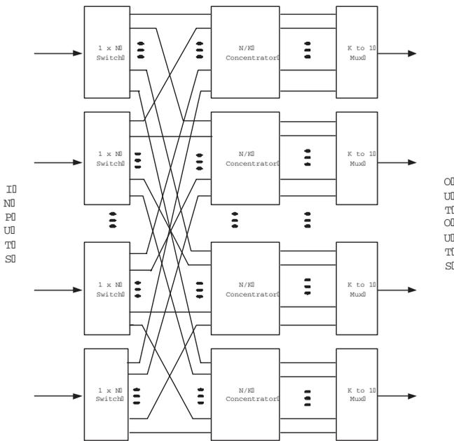
Fig. 9. An  $N \times N$  Knockout switch
