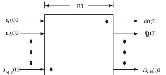
Fig. 2. An  $N$ -to-1 multiplexer with buffer  $B$
